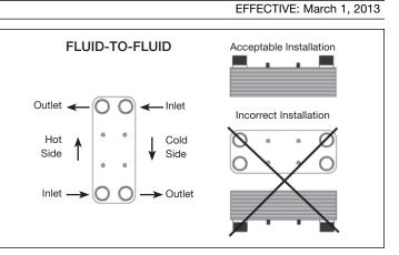
**Steam Applications –** Unit should be installed in a vertical position to ensure the condensate properly drains from the heat exchanger.
