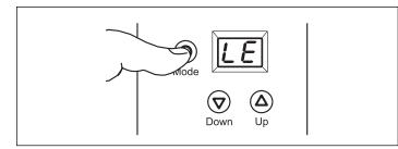
Press it once more to reach the current standard leak setting. Using the  $\triangle$  or  $\bigtriangledown$  buttons adjust the FloodBreaker to the desired setting. Hit the mode button Once more to save the setting. See Table 1 for code key.
