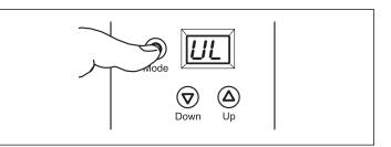
Press it once more to reach the current vacation leak setting. Using the  $\triangle$  button, adjust the FloodBreaker to the de-active setting (--).
