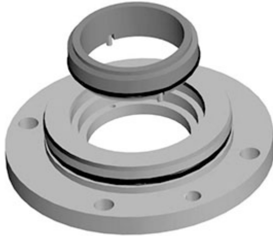
Figure 29: Mechanical seal seat and seal end cover (seal gland) assembly
