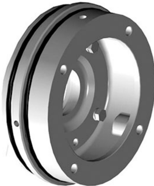
Figure 39: Seal end cover (seal gland) and O-rings installed onto seal body (stuffing box)
