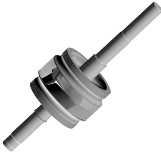
Figure 37: Impeller pressed onto shaft
