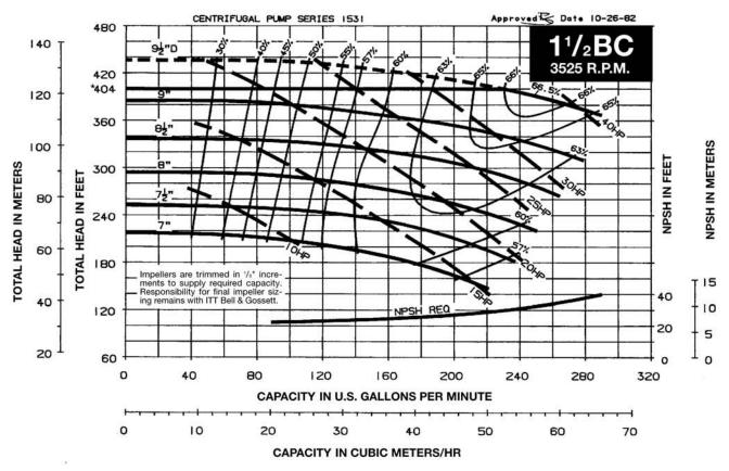
\*Operation above 404' will exceed the maximum pressure rating of the pump.
