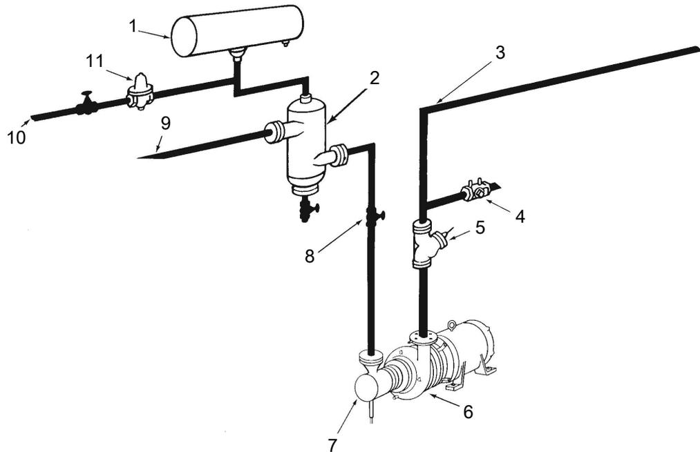
1. Compression tank (locate the compression tank on the suction side of the pump)
