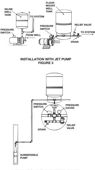
INSTALLATION WITH SUBMERSIBLE PUMP FIGURE 4
