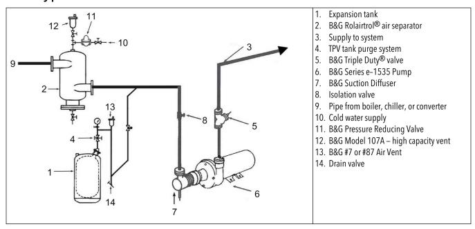
Do not install and operate B&G Series e-1535 pumps in closed systems unless the system is designed with these safety and control devices:
