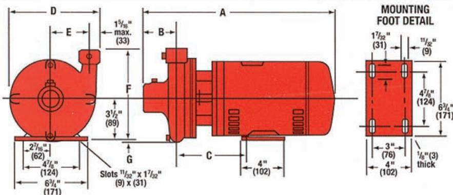
Bronze fitted Construction. Motors – Open Dripproof. Single Phase – Unit Number ending in "S", 115/230 Volt, 60 Cycle, 1 Phase. Three Phase – Unit Number ending in "T", 208-230/460, 60 Cycle, 3 Phase. All Single Phase Motors have built in overload protectors. **3500 RPM 175 PSI (12 bar) Maximum Working Pressure** Add "S" to pump number when ordering single phase pumps. Add "T" to pump number when ordering three phase pumps.
