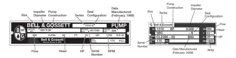
The nameplates above identify the pump as a Series 1510, size 5BC with a "-S" seal and bronze-fitted (BF) construction. The pump was furnished with a 9" impeller and a 20 horsepower, 1750 (1800) RPM motor. The serial number specifically identifies the pump for future reference. **DO NOT REMOVE THE NAMEPLATE.** It is important when ordering replacement parts to furnish complete nameplate data.
