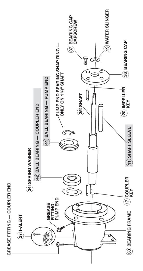
Note: Bearing lockwasher, bearing locknut and coupler end bearing cap (not shown) used on extra large bearing assembly only.
