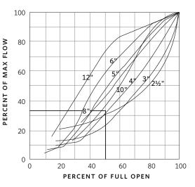
Record the size of valve and stem position using the Flow indicator scale (page 7). Calculate percentage of valve opening referring to table below:
