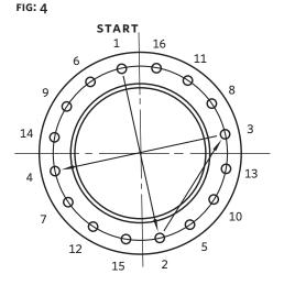
Tighten remaining nuts evenly, following bolting instructions (**FIG. 4**), so that the flange faces remain parallel. Flange bolts should be tightened to 70 ft/lbs torque minimum to assure firm metal-to-metal contact. When raised face flanges are used, there will be a gap between the faces of the outer diameter.
