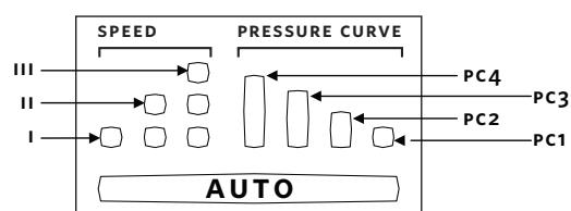
Lights on the display indicate the Control mode selected.
