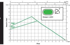
In proportional pressure mode (TRV), the circulator maintains a proportional pressure differential ( $\Delta p$ -v) in the system as heating load increases or decreases. Flow will change in relationship to the change in pressure differential. Selections options are Medium or High.
