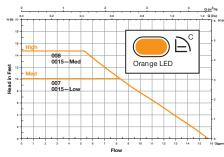
In constant pressure mode (ZV), the circulator maintains a constant pressure differential ( $\Delta p$ -c) in the system as heating load increases or decreases. Selections options are Medium or High.
